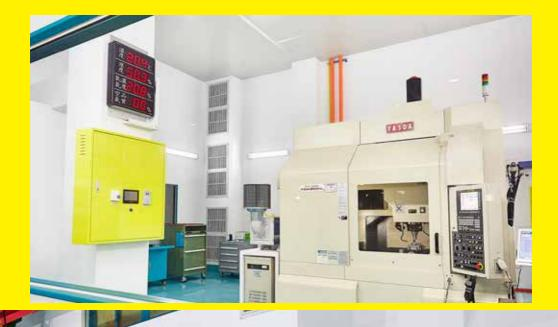
Precision machining in a temperature-controlled room (Micron-level accuracy)
